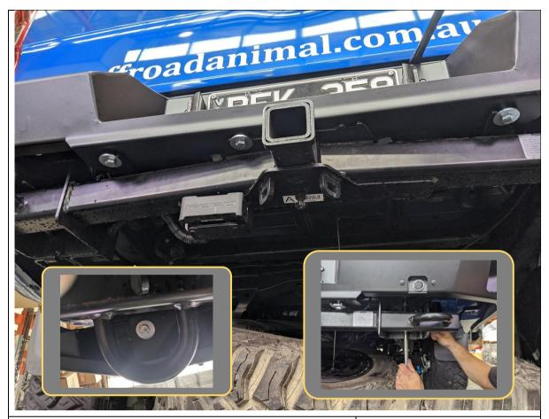
36. Secure Offroad Animal Bar to factory tow bar using M10x30 Bolts, M10 Large washers and M10 nuts in original factory locations.
