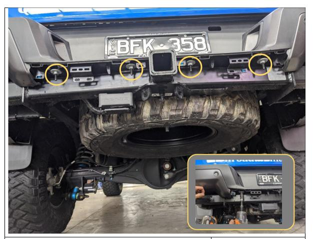
4. Remove 4x M8 nuts side securing the bottom edge of the rear bar. to the Chassis. Due to length of the studs use a deep socket for easy removal.
